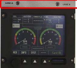
Schritt 5 Fuel Pressure min 3.0 bar
